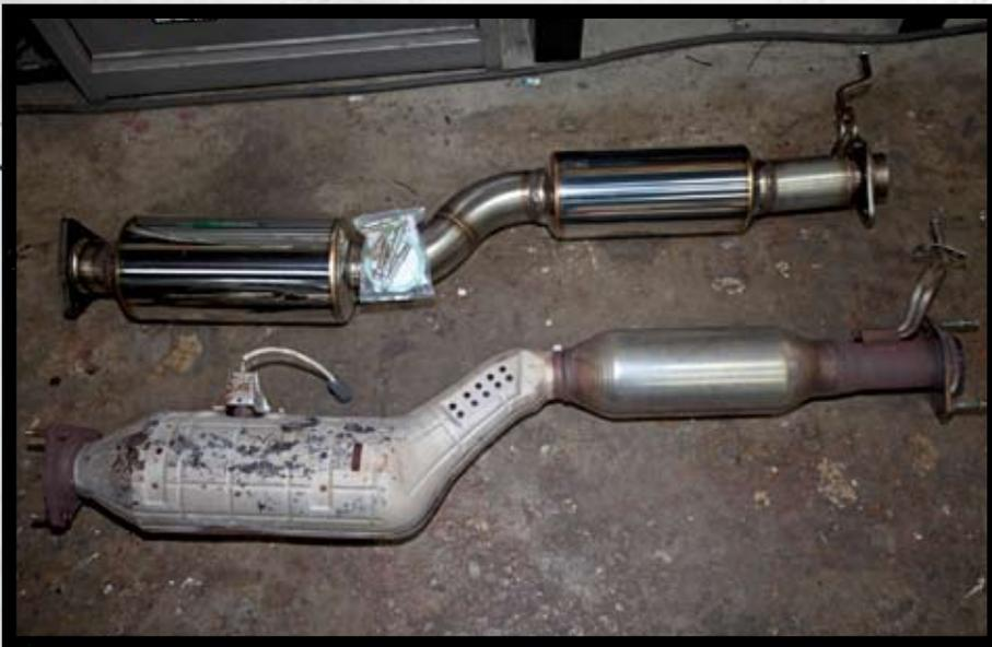
Racing Beat's resonated race pipe deletes the OE cat, but keeps sound level very close to factory quiet thanks to the two large resonators.
