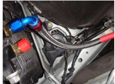
Connect oil line to the adaptor installed on the OUTER connection on the cooler.
