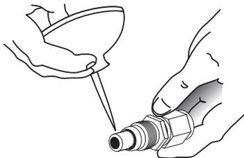
3. Lubricate the inside of the hose, the cutter threads and the socket threads with Earl's assembly lube or engine oil. Place the nipple in a vise.
