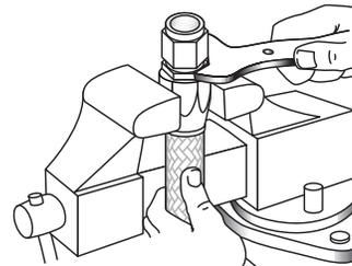
5. To complete the assembly it doesn't matter whether the nipple or the socket is held in the vise. Holding one or the other in the vise and using a suitable wrench on the other, tighten the socket onto the cutter threads until the socket is with in .060" of bottoming on the nipple. Do not use an adjustable or over-size wrench or you will damage either the nipple or the socket.
