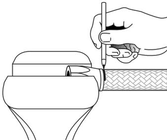
2. Place the socket in a vise and insert the end of the hose into the socket until the hose butts against the bottom of the threads provided for the cutter. Gently pull the hose back until there is a 1/16" to 1/8" gap between the end of the hose and the bottom of the threads—mark hose at bottom of socket with a felt pen so that you can detect any tendency of the hose to be pushed out as you complete the assembly.
