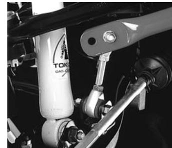
7. Torque the attachment clamp bolts to 17 ft lbs. If using the stock end links, torque the link bolts to 32 ft lbs.
