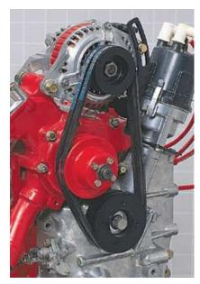
**Double Sheave Alternator** & Main Drive Pullev
