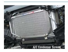
Note: In late 2005, Mazda started supplying the RX-8 with a small lower "half-screen". Although this screen appears to offer adequate protection, if you prefer 100% protection coverage you can remove the factory screen and install the Racing Beat unit.
