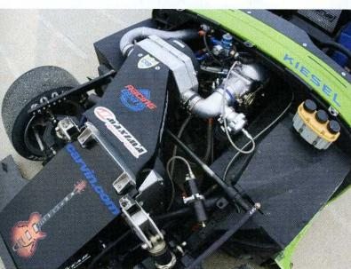
(ABOVE) Improvements to the intake manifold, intercooler and turbo (TOP LEFT) have improved drivability and power output this season, all while helping to reduce the weight on the front of the car. (TOP RIGHT) A new rear spoiler design aids high-speed stability and helps keep the back tires planted.
